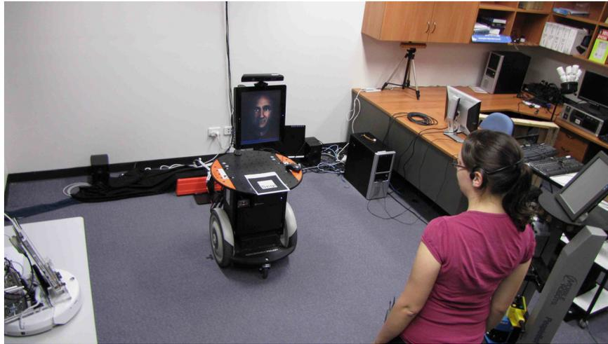
Fig. 2. Segie—the software-rendered head is displayed on an LCD screen affixed to a Segway unit.
